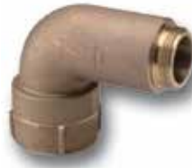
635 90° Continuous Swiveling Elbow FEMALE NPT x MALE NH or NPSH • Full 2" (51 mm) waterway with cast-in turning vane # 1 1/2" or 2" female x 1 1/2" male (38 or 50 x 38 mm) 4 5/8" length # 2 1/2" female x 2 1/2" male (65 x 65 mm) 5" length
