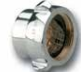
338 Suction Lug Adapter with Strainer FEMALE NPT x FEMALE SWIVEL ◇ 1 1/2" NPT x 1 1/2" NH (38 x 38 mm) ◇ 2 1/2" NPT x 2 1/2" NH (65 x 65 mm)
